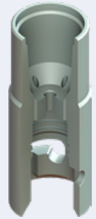
TEMPORARY CAP RUNNING/RETRIEVAL TOOL
